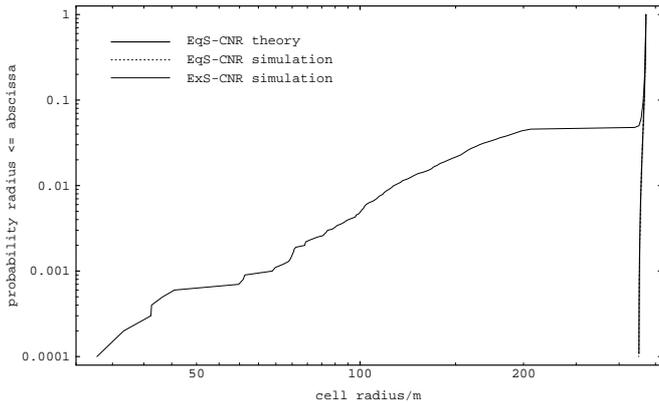
Fig. 8  $F_P(\rho)$  for Constrained Non-Roaming terminal distribution
