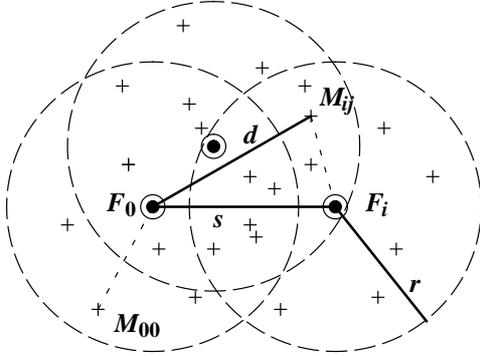
Fig. 2 Non-Roaming terminal microcell distribution model
